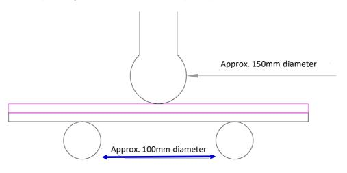
• Pipes – Pressing / rolling should be performed so the weld overlay is perpendicular to the flow of material through the pipe.
